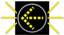
The use of flashing yellow left turn arrows is a relatively new national standard. Only three states are not using the flashing yellow arrows at all. In 2008, Maryland had planned to require that all new signals have flashing yellow arrows. But their new state MUTCD prohibits the flashing yellow arrow in favor of the flashing red arrow that Maryland has used for years.
